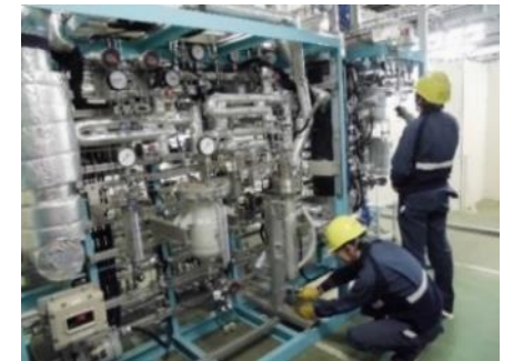
Membrane reactor of methanol synthesis (pilot test)
