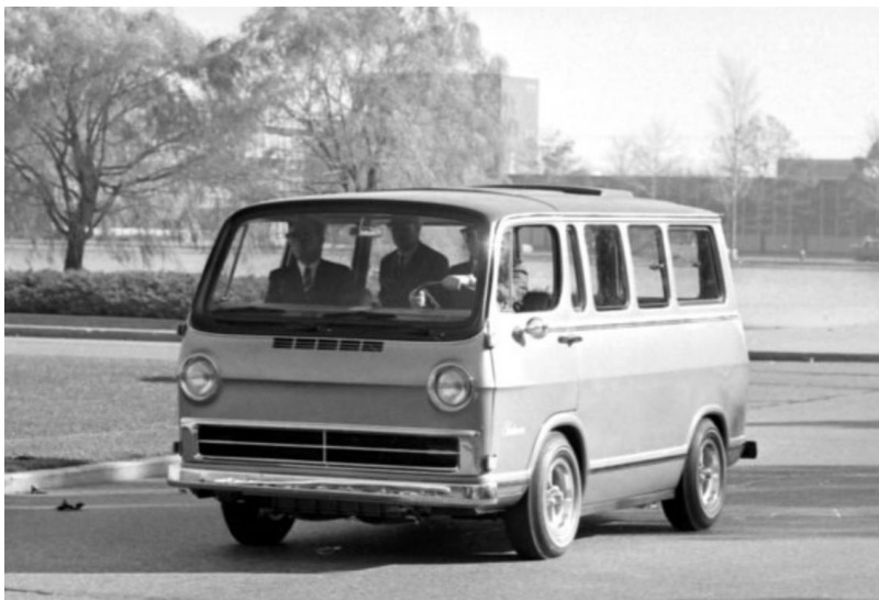
Figure 6, the Chevrolet Electrovan was powered by fuel cell technology spun off by NASA's Moonshot programme, photo by John Lloyd (CC-BY 2.0).
