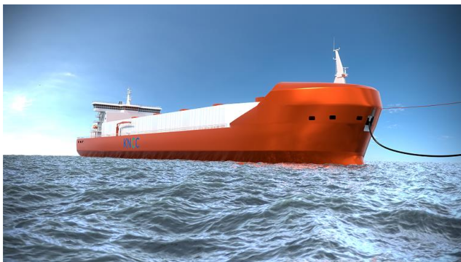
Image of liquefied CO 2 carrier with bow loading system from NYK website
