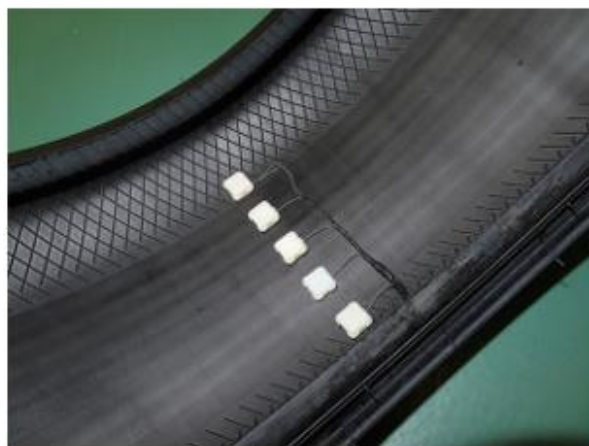
Power generation device installed in the tire
