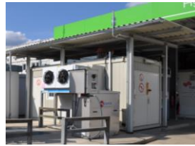
GH 2 test stand up to 1000 bar with climate chamber
