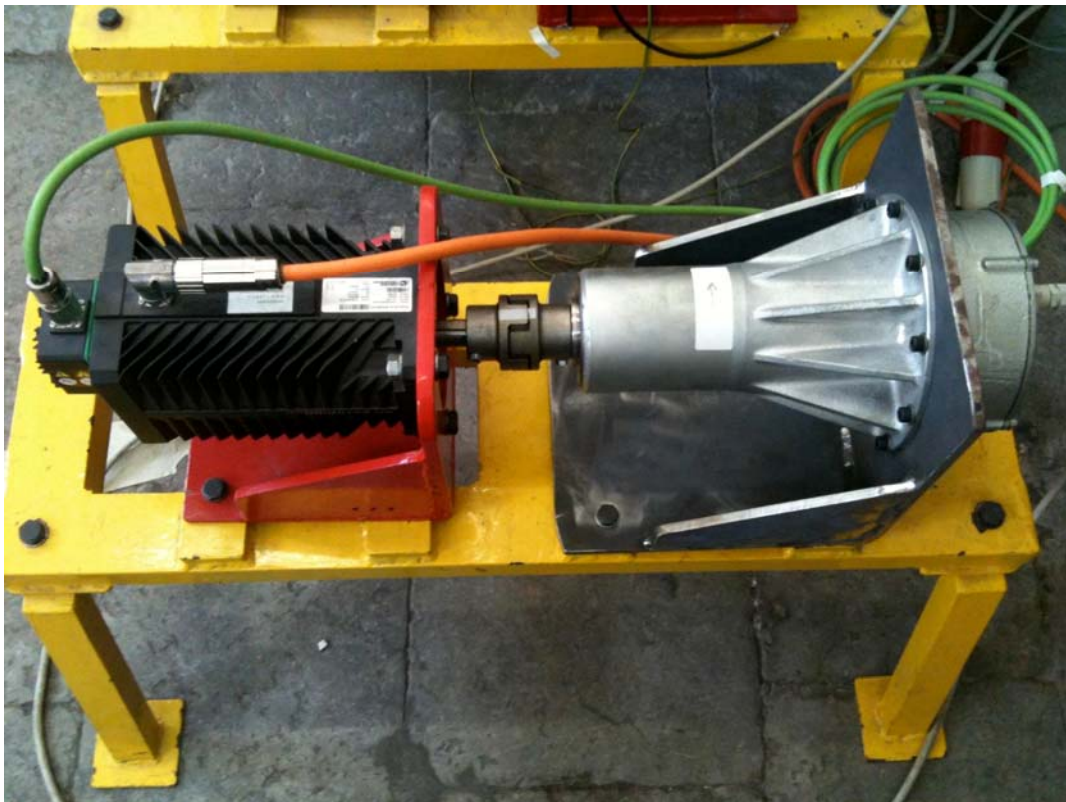
Micro-WECS: turbine emulator and generator
