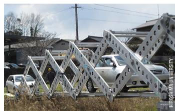
At a recent test, the largest folding bridge developed to date was deployed across a small stream and tested with passenger vehicles. Hiroshima University
