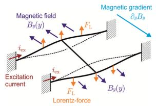
Working principle of the magnetic gradient sensor.
