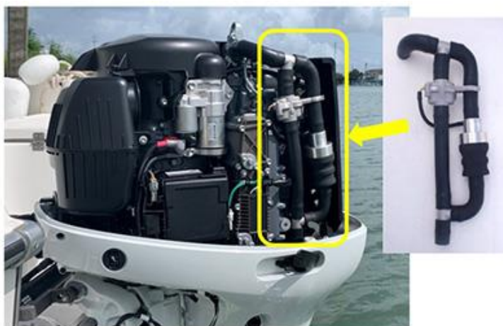
Outboard motor installed with Micro-Plastic Collecting Device
