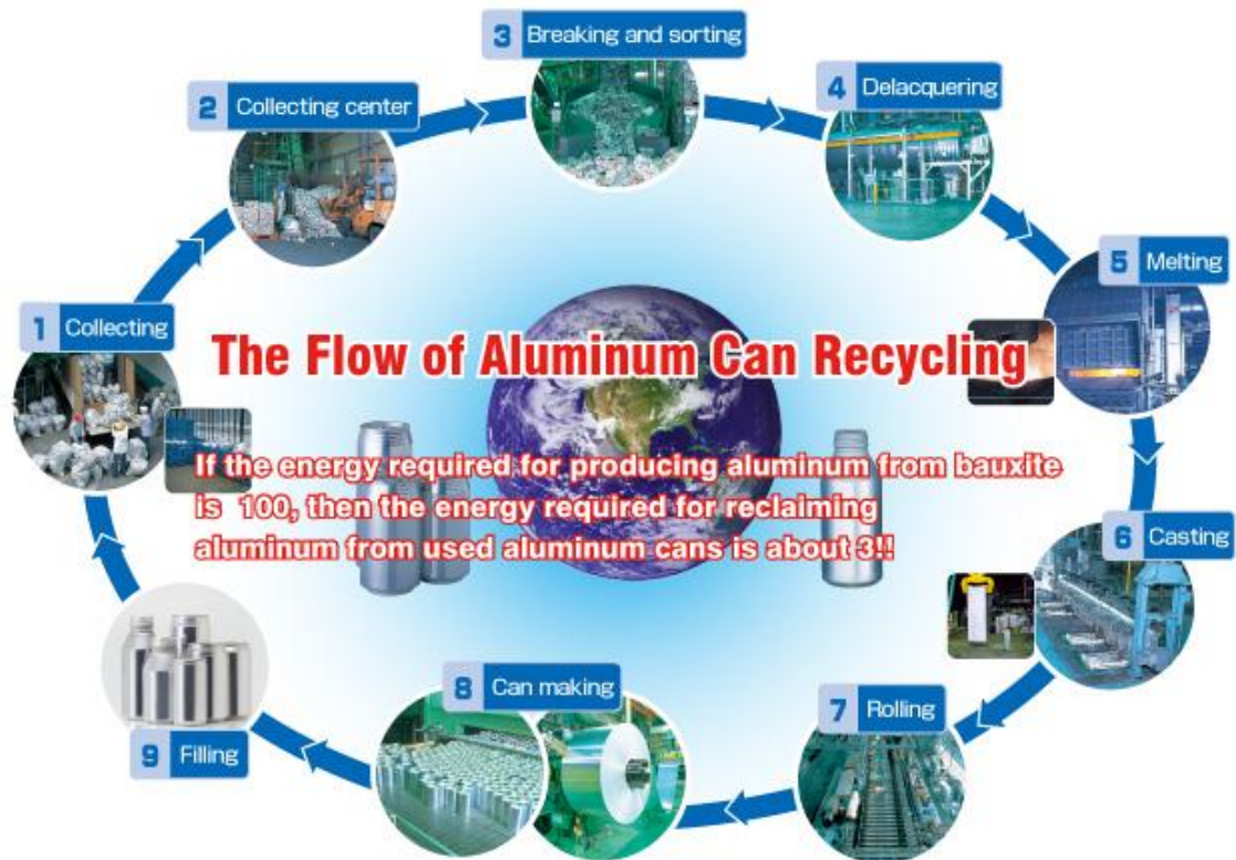
Figure 17: Mitsubishi Material Corporation, Aluminum Recycling Flow
